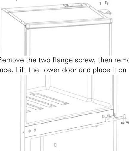
4. Remove the two flange screw, then remove the middle hinge that hold the lower door in place. Lift the lower door and place it on a padded surface to prevent scratching it.
