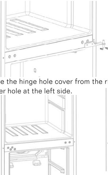
5. Remove the hinge hole cover from the right holes as illustrated and transfer them to the uncover hole at the left side.
