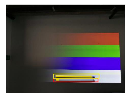
There are two yellow bars in the bottom center of the screen and you can adjust it to get better picture. The Red, Green, Blue & White block of the above picture should be as smooth as possible and No grey scale should be visible.
