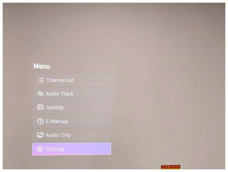
(3) Move and "ok "button on RC to select Setting-Sound-Speakers-Balance
