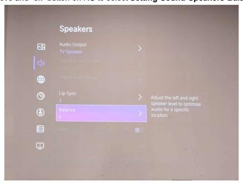
(4) On the **Balance**, input figure 1->9->6->9 in sequence on RC.
