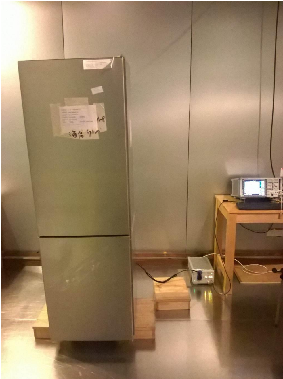
Figure 10 Mains conducted disturbance voltage test setup
