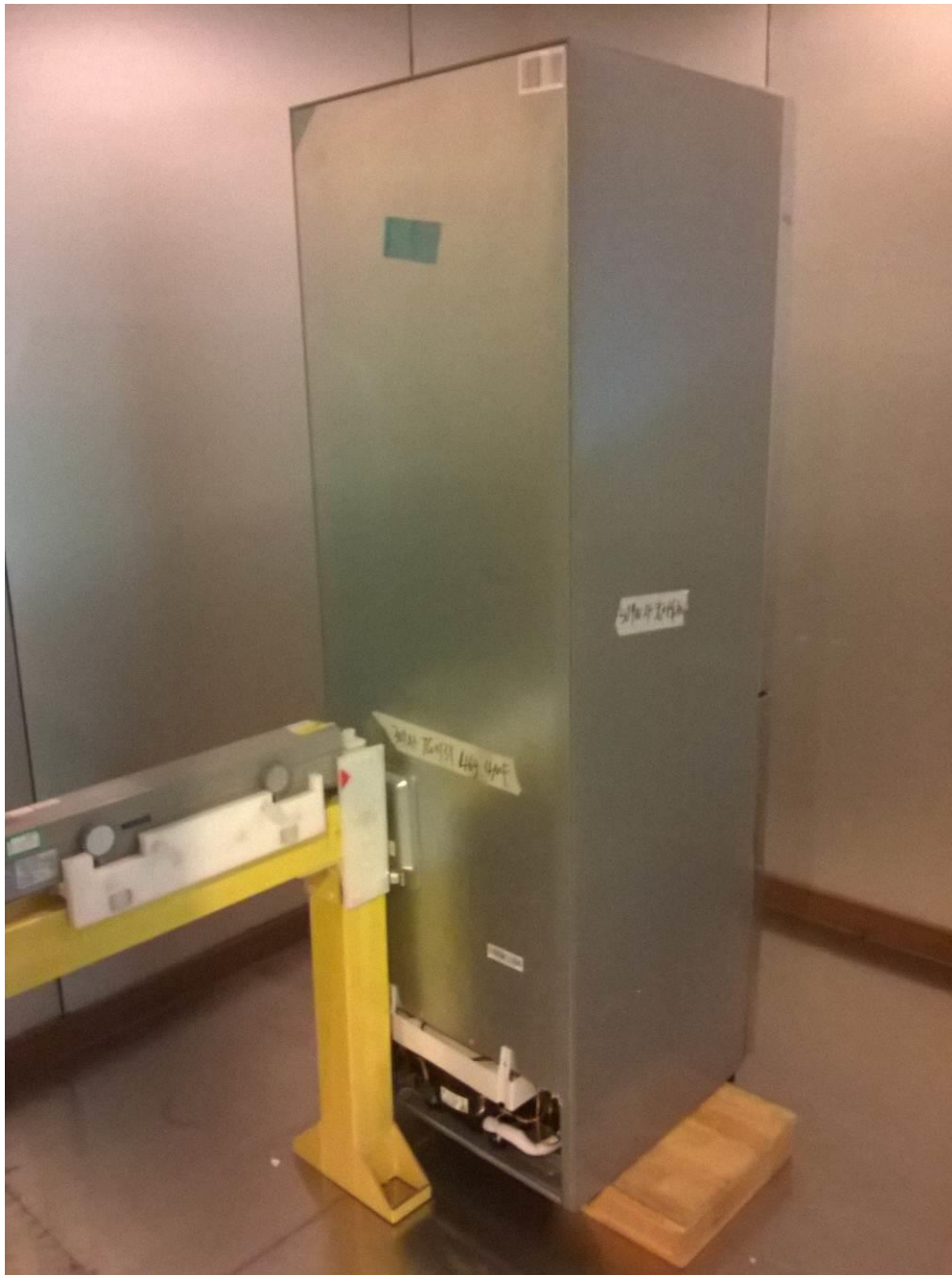
Figure 11 Disturbance Power test setup
